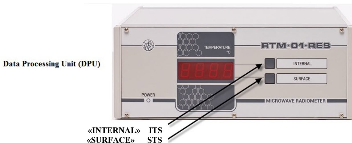
Fig.1 Data Processing Unit (DPU)
